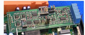
Removable calibration board with surface mounting technology (smt)
