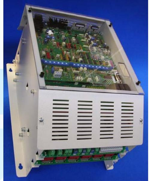
Galvanic isolation, also in armature feedback, with compensation Rxl. Adjustable speed relay (0.5 to 120%). Thermal overload prealarm relay (I2t). Electronic thermal images. Provision for setting (1.5x In per 30 s.) and disabling overload. Commands for controlling references and functions, with LED signalling handled by the PLC or process controls. Analog current and speed outputs. Differential proportional amplifier, configurable by the
